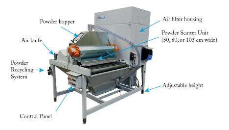
**Excess powder removal.** With vibrations, air pressure, vacuum and a combination of different antistatic technologies, the WPA clean the excess powder of the heat-transfers with ease. This combination of technologies ensures a steady and streamlined production process with a high quality end-product.
