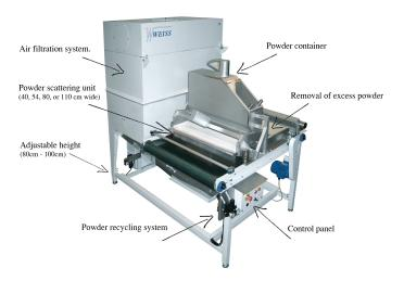
**Excess powder removal.** With vibrations, air pressure, vacuum and a combination of different antistatic technologies, the WPA clean the excess powder of the heat-transfers with ease. This combination of technologies ensures a steady and streamlined production process with a high quality end-product.
