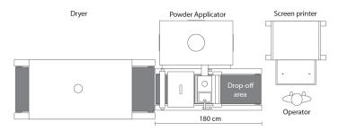
If you produce your screen prints automatically on a conveyor, there is no need of a drop-off area and the conveyor belt is shortened to a length of 130 cm.
